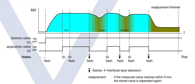
Start: when opening bottom valve V1, switch the corresponding digital inputs (D1-D3) to 1 (+24 V) ID flashes: interfacial detection on; ↓/↓ flashes interfacial layer detected; V2 separation valve closes (relay 2 = deenergised)
