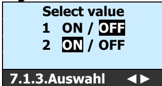
1. Using the **▲▼◀▶** buttons the output relay or open collector transistor output (NPN) is switched over to 1 or 2
