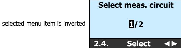
After pressing the **ok** button the display changes to the menu of the selected measuring circuit (1). 2.4.1.
