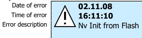
1. press **ok** button more than 2 seconds, the error is confirmed and the display changes back to last active menu point
