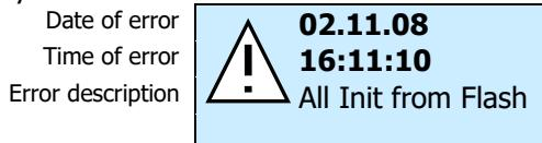
1. press **ok** button more than 2 seconds, the error is confirmed and the display changes back to last active menu point
